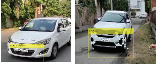
Figure 2. Bounding boxes detecting and tracking in various videos using faster RCNN and KLT.
