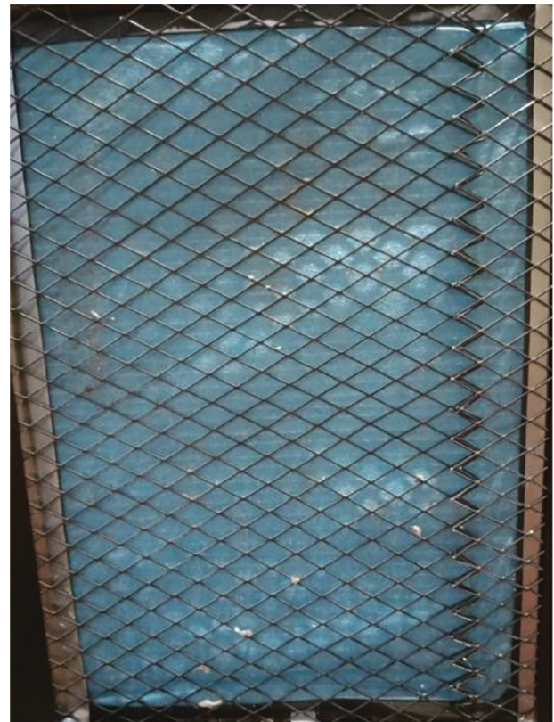
FIGURE 6 | Testing of the product in a 60 square meter room with 26 people and used for 6 h. Presence of dust and other particles are seen in the 1st layer of filter which is the non-woven.
