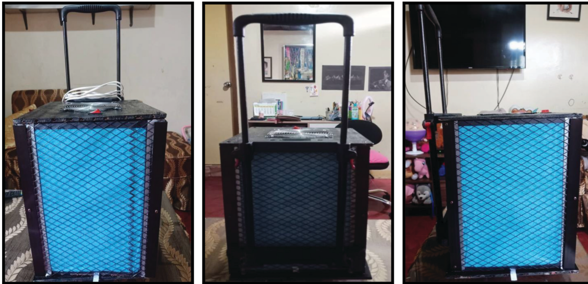
FIGURE 4 | The actual project. Eco air purifier using air filter with activated carbon.
