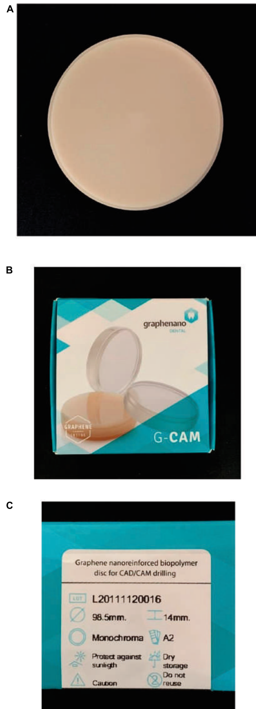
FIGURE 2 | (A) CAD/CAM PMMA resin reinforced with Graphene blank. (B) Manufacturer packaging of CAD/CAM PMMA resin reinforced with Graphene blank (front cover). (C) Manufacturer packaging of CAD/CAM PMMA resin reinforced with Graphene blank (back cover).
