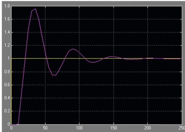
FIGURE 4 | Theoretical data of the tank level vs. time—ZN.
