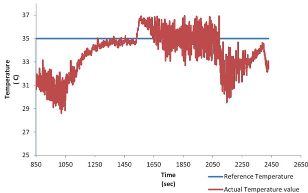
FIGURE 5 | Hot water (HW) to temperature—ZN technique.
