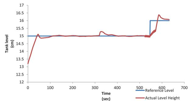
**FIGURE 2** | Cold water (CW) to tank level—ZN technique.
