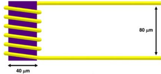
FIGURE 6 | A solenoidal microcoil for magnetic stimulation with an interior (purple) consisting of iron-gallium-boron, which has a relative magnetic permeability of nearly 1,000. From Khalifa et al. (33).
