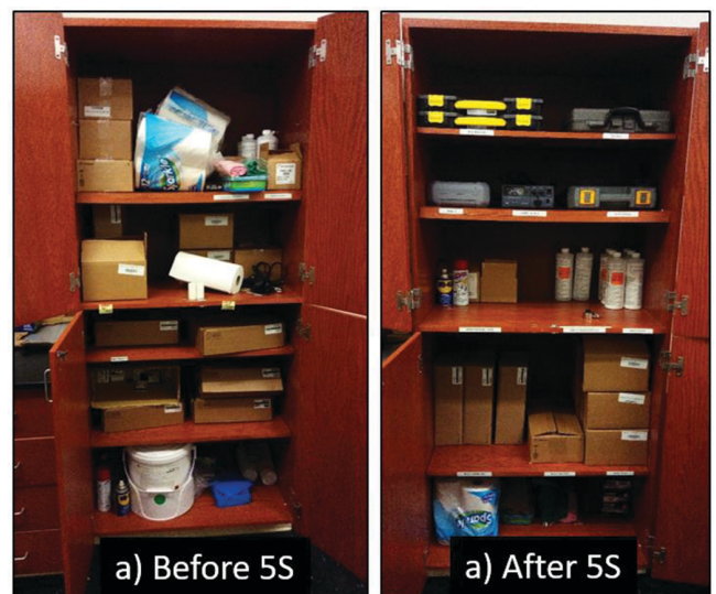
FIGURE 8 | 5S implementation in cabinet area.
