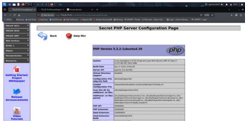
FIGURE 21 | Exposure of outdated hypertext preprocessor (PHP) version (5.3.2).
