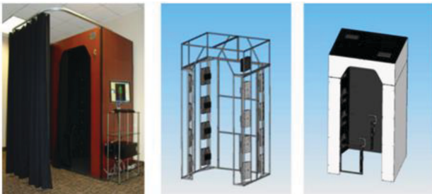
FIGURE 1 | Size stream 3D body scanner includes 14 sensors.
