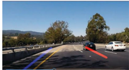
FIGURE 14 | The presence of shadow patterns can result in the inaccurate detection of lane lines.
