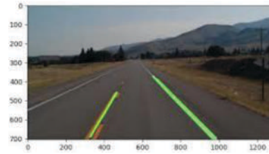
FIGURE 2 | The lane-line RTRD algorithm detects and identifies the boundaries of the detected lane lines.
