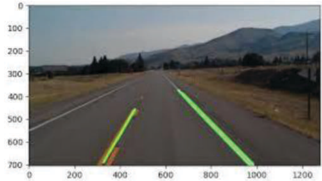
FIGURE 11 | The picture contains solid yellow and dotted white lane lines segments. The lane lines are in a left-turned lane, and there are no cars in the image.
