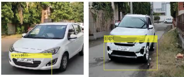
FIGURE 2 | Bounding boxes detecting and tracking in various videos using faster RCNN and KLT.
