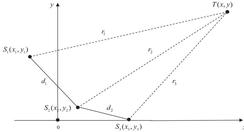
FIGURE 2 | Geometric schematic diagram of a planar arbitrary three-station positioning array based on mixed equations.
