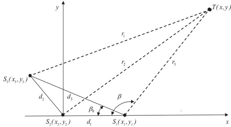
**FIGURE 1** | Schematic diagram of a planar arbitrary three-station positioning array with known baseline angles.
