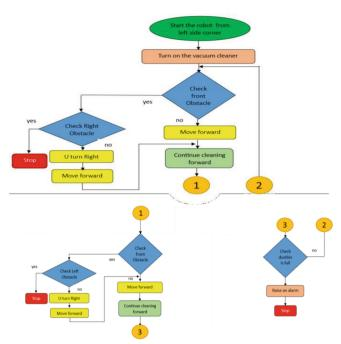
In operating conditions, the autonomous vacuum cleaner will check for obstacles: if no obstacle is found, the cleaner will move forward. An obstacle is detected by the ultrasonic sensor by transmitting ultrasound from the transmitter of the ultrasonic sensor.
