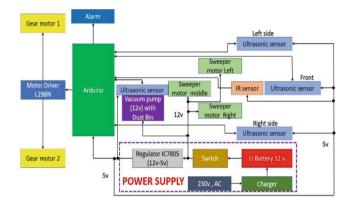
In this block diagram, there are three ultrasonic sensors are connected to the Arduino Uno microcontroller. The transmitting and receiving signals are given through the microcontroller. The sensors are used for obstacle detection.
