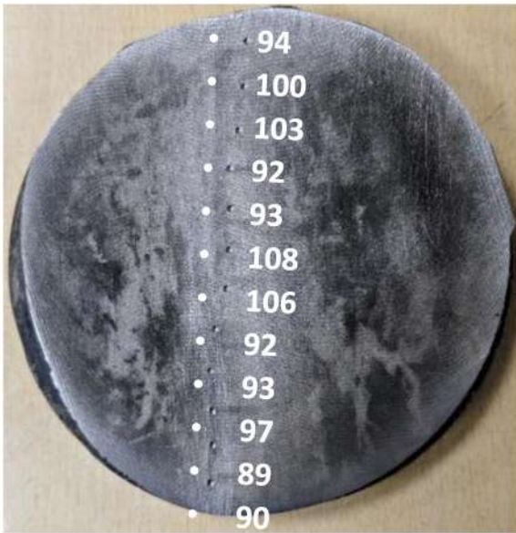
FIGURE 4 | Brinell hardness of the hook shows no systematic variation from surface to core.
