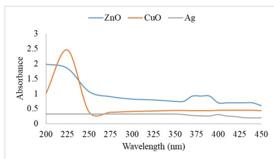
**FIGURE 2** | UV-Vis profile showing absorption peaks of ZnO NPs, CuO NPs, and Ag NPs.
