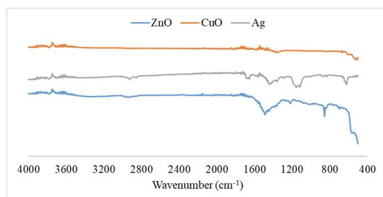
**FIGURE 3** | Fourier-transform infrared (FTIR) spectra showing functional groups of ZnO NPs, CuO NPs, and Ag NPs.
