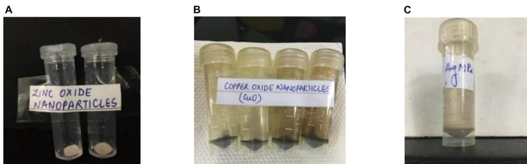
**FIGURE 1** | Synthesized (A) ZnO NPs; (B) CuO NPs; and (C) Ag NPs.
